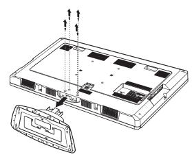
3 Attach the included TV base cover to the TV base to prevent debris from entering your TV after it is mounted on the wall.
